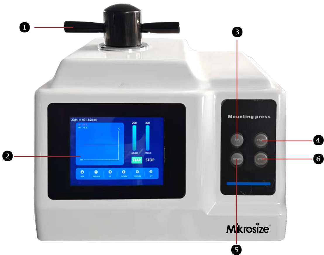
1. Upper mold cover 2. Display screen 3. Up button 4. Start button 5. Down button 6. Stop button
